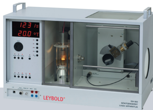
X-ray apparatus (554 800) with Bragg crystal and counter tube in operation.
